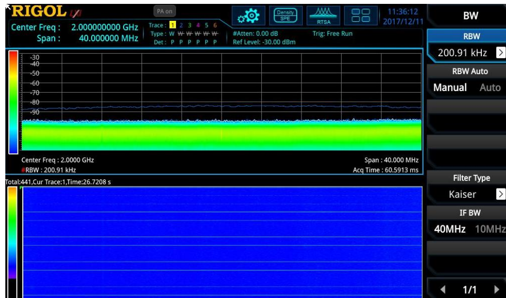
Figure 9: Measurement of a pulse of 25 nsec. (period: 1 sec.) with amplitude of -35 dBm. Not all pulses are captured. Amplitude is wrong amplitude.
