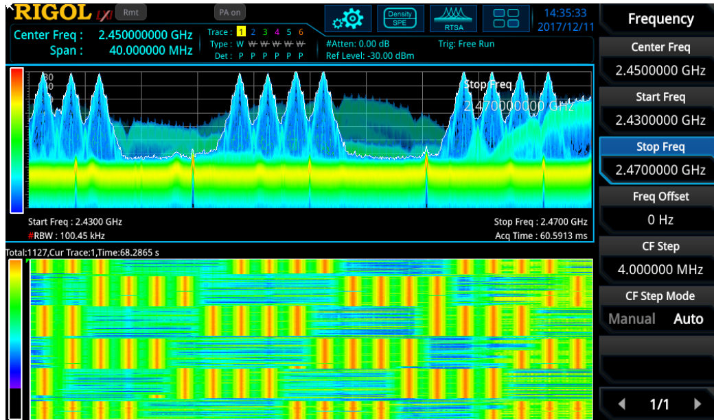
Figure 12: Bluetooth signal measured with density spectrogram
