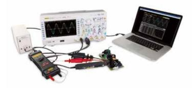
Power supply is an important component of electronic devices. The quality of power supply will have direct influences on the electronic devices. During the design and manufacture of power supply, performance testing becomes more and more important.
