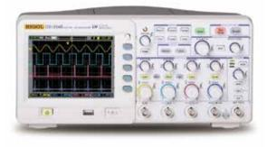
DS1000B series products are four-channel plus an external trigger oscilloscopes which can capture multi-channel signals at the same time to meet the industrial needs.
