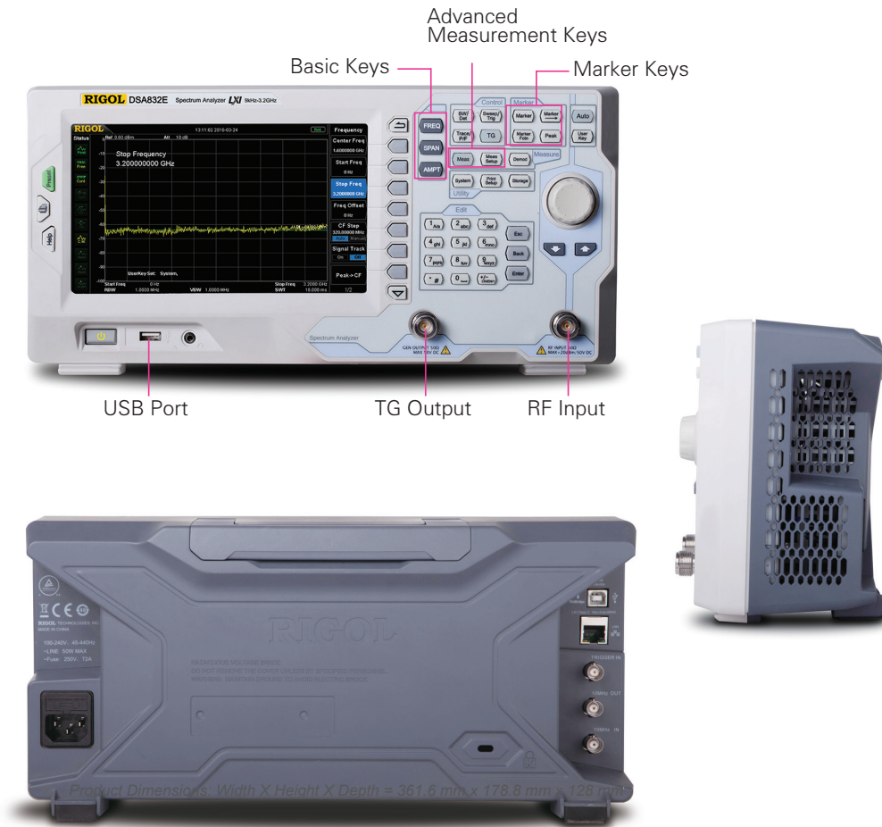
Product Dimensions: Width × Height × Depth = 361.6 mm × 178.8 mm × 128 mm
