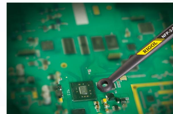
NFP-3-P3, a near-field probe which resolution is 5 mm. It is applicable for the detection magnetic field on surface. For example, the detection of the magnetic field produced by the wire, cable, metal surface, connectors, electronic components, and component joints.
