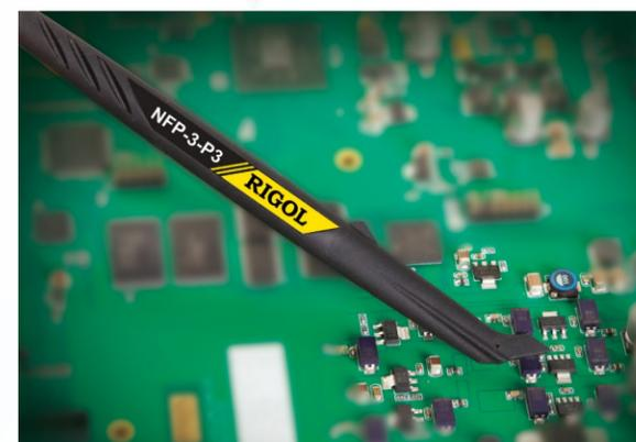
NFP-3-P4, a near-field probe which resolution is 2 mm. It can detect the vertically emitted electromagnetic field. It is applicable for the detection of magnetic field where current loop exists. For example, electromagnetic field testing for PCB wiring, magnetic field testing for IC pins area etc
