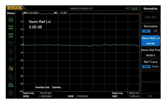
The trace should now be a flat line at the top (0dBm) of the display. This indicates that any reflections and losses are "normalized" and removed from the trace.
