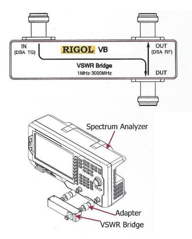
If you are using another direction coupler or bridge, please see the connection instructions for the specific model you are using to ensure proper connections.
