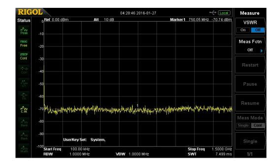
• Press FREQ > Stop Freq > Use Keypad or scroll wheel to enter stop frequency and select units.
