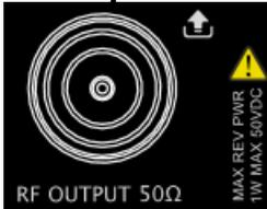
When the backlight of **RF** lights on, this connector is used to output RF signal and RF sweep signal.
