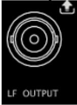
When the backlight of **LF** lights on, this connector is used to output LF signal.
