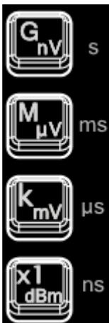
Used to set the unit of the parameter.
