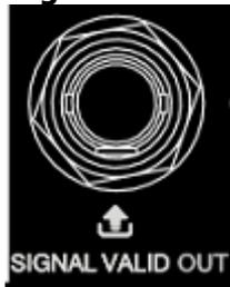
When the RF output frequency or amplitude is modified, after a certain response and processing time, the internal circuit of the instrument outputs RF signal with specified frequency and amplitude via the RF output connector on the front panel. During this process, the **[SIGNAL VALID]** connector outputs a pulse sync signal, indicating that the RF output signal is valid.
