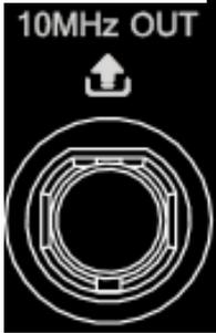
It is used to output the internal 10 MHz reference clock signal used to synchronize the generator with other instruments. For more information about the output clock signal specification of this connector, please refer to *DSG3000B Data Sheet*.
