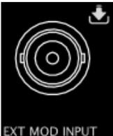
When the modulation source of AM, FM and  $\phi$ M is external, this connector is used to input the external modulating signal.
