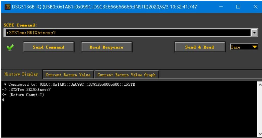
Figure 3-2 Read and Write Command via USB
