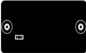
OCXO is an oven-controlled crystal oscillator. It is a frequency reference source with higher temperature stability.
