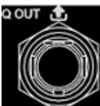
It is used to output the Q (Quadrature Phase) components of the I/Q modulation of the built-in baseband generator.
