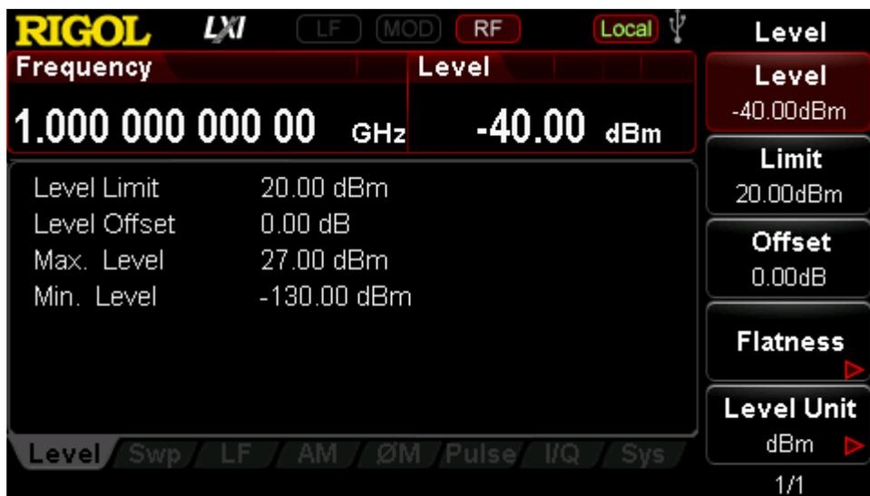
Figure 4-1 Parameter Setting Interface of RF Signal Output
