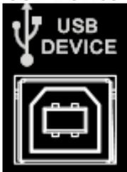
The instrument complies with USBTMC class protocol. This interface is used to connect to a PC for remote instrument control.
