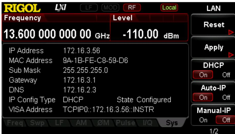
Figure 2-3 To Set the LAN Parameters
