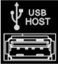
This input is used to connect the USB storage device to update the system, store system states and sweep lists.
