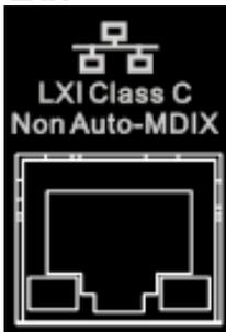
The instrument complies with LXI Device Specification 2011 standard, and supports WebServer, Socket and other remote control modes. This interface is used to connect the PC or network for remote instrument control.
