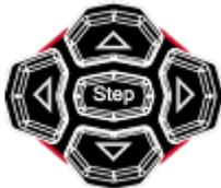
When setting the parameters, **Step** is used to set the step of the parameter currently selected.
