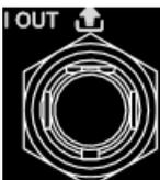
It is used to output the I (In-Phase) components of the I/Q modulation of the built-in baseband generator.
