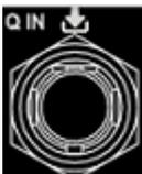
When I/Q modulation type is "external", it is used to input the Q (Quadrature Phase) modulating signal of I/Q modulation.
