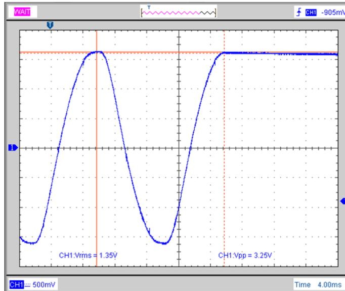
**Figure 7. Example of Sine Wave disconnected on peak.**
