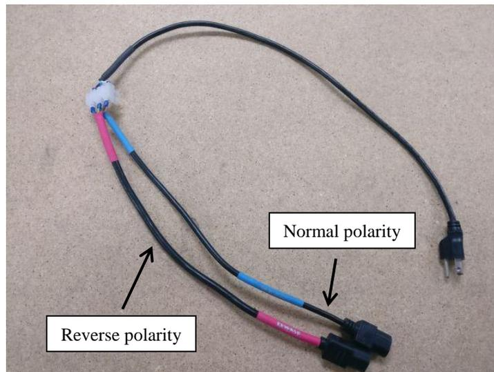
**Figure 6. Normal connection (Right), Reverse connection (Left).**
