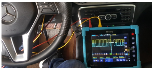
Power CAN bus communication
