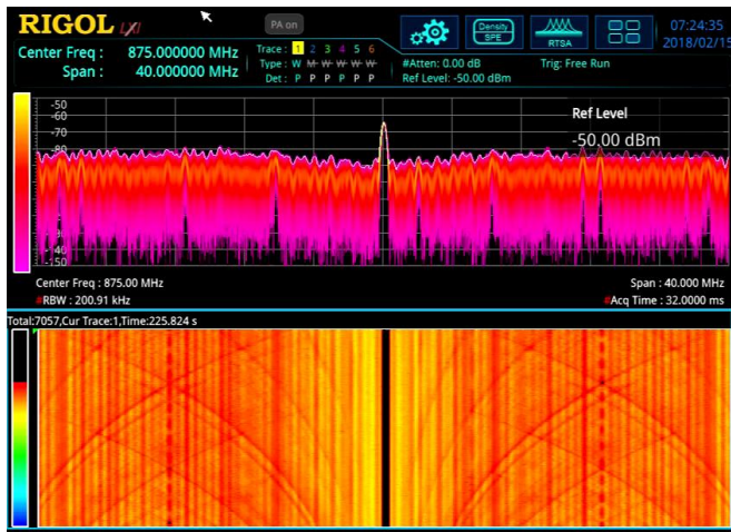
Figure 9: Debugging emissions with the density display (top) and the spectrogram waterfall chart (bottom)
