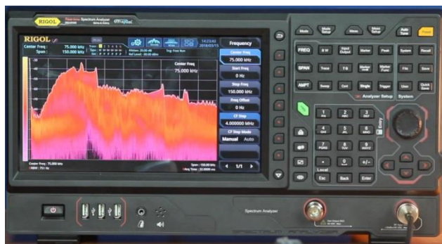
Figure 5: Conducted Emission profile of an LED light fixture
