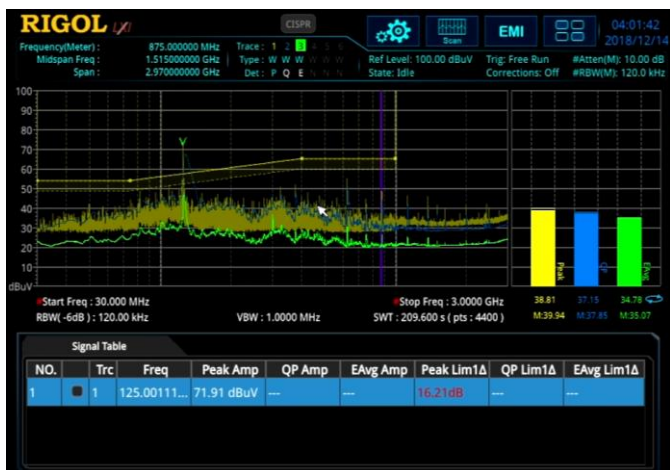
Figure 7: EMI Mode using limits, multiple detectors, and meters on a RSA Series Real-Time Spectrum Analyzer
