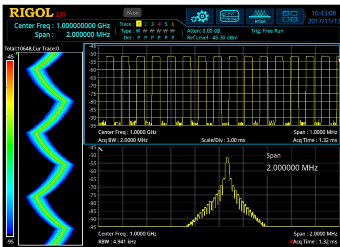
Figure 10: Debugging with a combined view of the spectrum (bottom), power over time (top), and spectrogram (left)
