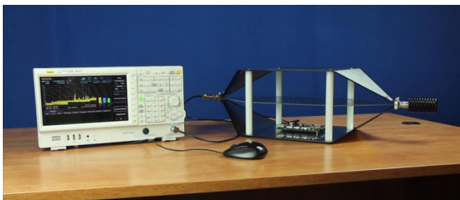
Figure 8: A TEM Cell for repeatable radiated emissions testing
