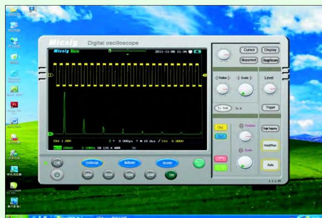
The functions of scopesuite include updating, real time control, measurement, storage, dynamic display, record, data analysis
