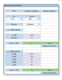
Workers should wear hearing protectors if the noise or sound level at the workplace exceeds 85 decibels. The selection of hearing protectors depends on a noise level in the working environment. Therefore the selection of suitable hearing protector should be based on noise measurement.
