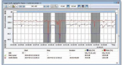
The Supervisor software gives tools to simulate hypothetical situations in which the noise differs from that which was measured. When selecting a data block it is possible to shift the data up or down for any given dB value. It is also possible to simulate a situation where noise is equal to a given dB level or completely removed from time history. The altered data is recalculated automatically and both the original and recalculated results are shown so as to answer the question "What if".
