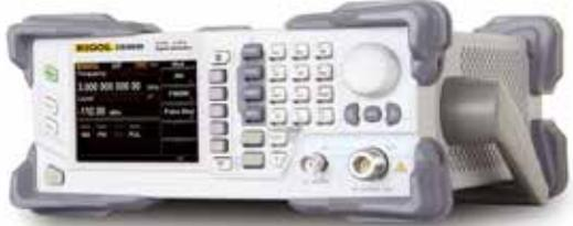
DSG3000 is a high performance RF signal generator which ranges from 9 kHz to 3 GHz/6 GHz. It is designed for the customers who works in the application filed of Wireless Communication, Radar test, Audio/Video Broadcasting, General Purpose, Education, Consumer Electronics etc. DSG3000 provides variety of analog, digital IQ and pulse modulations with high quality signal and stable specifications. It is a desirable choice for replacing of import products.
