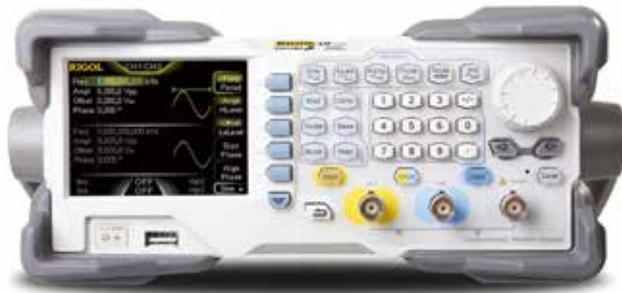
DG1000Z series function/arbitrary waveform generator is a multi-functional generator that combines many functions in one, including Function Generator, Arbitrary Waveform Generator, Noise Generator, Pulse Generator, Harmonics
